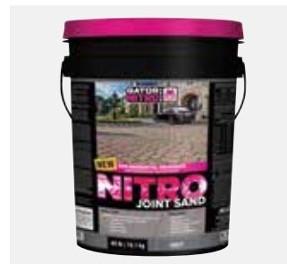
GATOR NITRO SAND The ideal air cure, permeable jointing material. It is a ready-to-use mixture of calibrated sand and proprietary resin formula which cures when exposed to air, hardening from top to bottom of the joint. The product can be installed in wet or dry weather.
