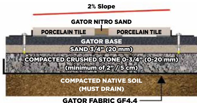
GATOR NITRO SAND The ideal air cure, permeable jointing material. It is a ready-to-use mixture of calibrated sand and proprietary resin formula which cures when exposed to air, hardening from top to bottom of the joint. The product can be installed in wet or dry weather.
